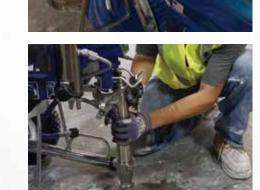
**ProConnect™ 2** This next-generation pinless design of Graco's ProConnect Pump Removal and Installation System makes it easier and faster than ever to replace the pump in seconds.
